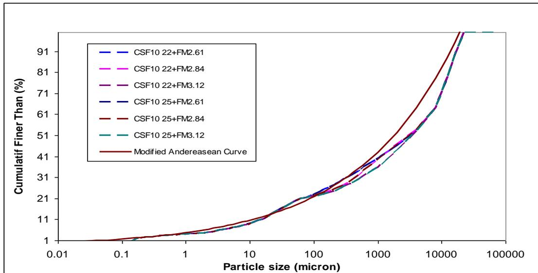
Figure 3: Particle size distribution of concrete mixtures series containing CSF combined with aggregates and modified Andreason model curve for  $q = 0.28$
