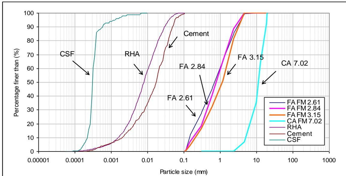
Figure 1: Particle distribution of fine aggregate and coarse aggregate
