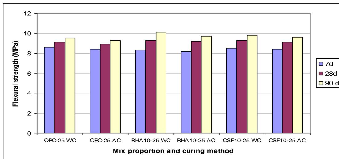
Figure 7: Flexural strength of high strength concrete
