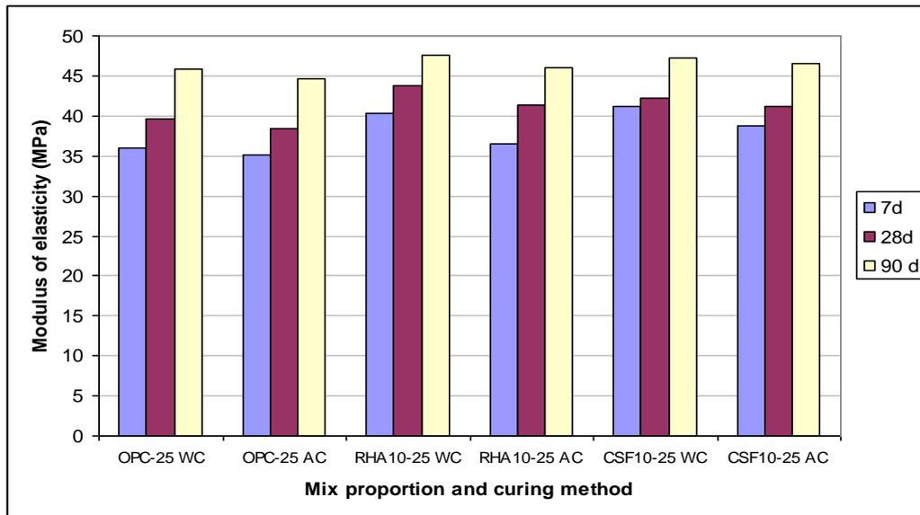
Figure 8: Static modulus of elasticity
