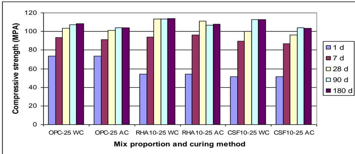
Figure 5: Compressive strength of high strength concrete
