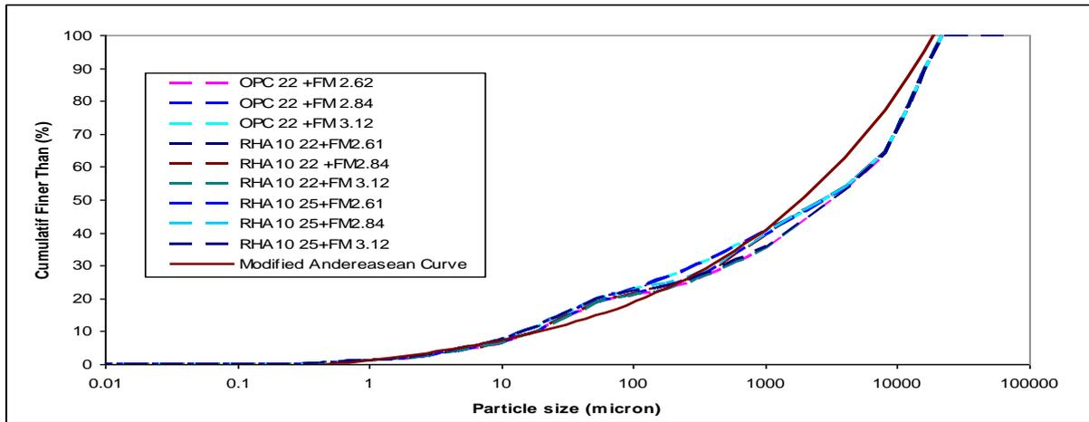
Figure 2: Particle size distribution of concrete mixtures series containing OPC and RHA combined with aggregates and modified Andreason model curve for  $q = 0.28$
