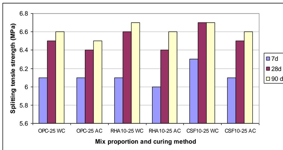
Figure 6: Splitting tensile strength of high strength concrete
