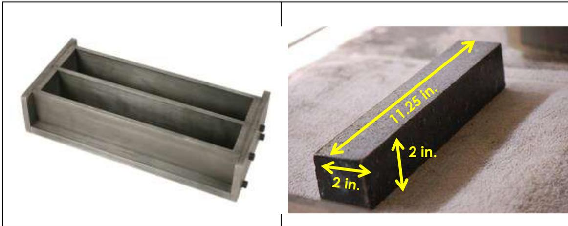
Figure-1 MCPT specimen and mold
