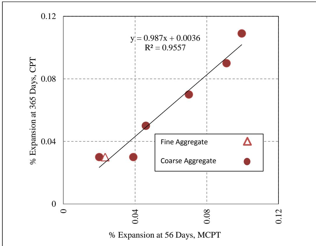
Figure -3: Correlation between the 56-Day MCPT data and the 365 Day CPT data excluding aggregates with very high expansion values ( $> 0.200\%$  at 56 days).
