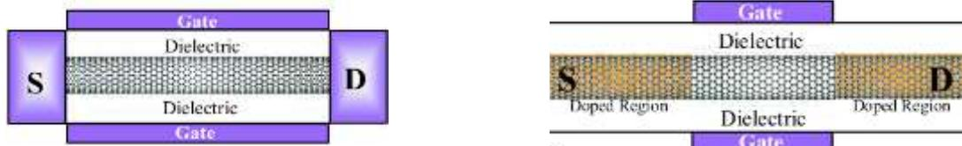
Fig. 2 a) Schottky Barrier CNTFET, b) MOSFET-like CNTFET.
