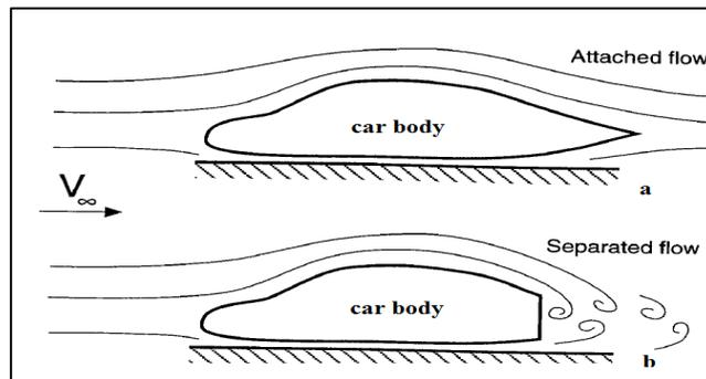
Reducing separation pressure drag by keeping the flow attached will result in a greater skin friction drag. Interference drag will always exist as it is impossible to produce a car shape that does not have appendages. Pressure drag contributes a large percentage in total aerodynamic drag where viscous, induced and interference drag contributes very small percentage but have to be considered important for race car design.
