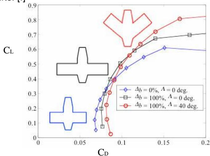
**Fig 10:** CL vs. CD for conventional and morphed wings [1]
