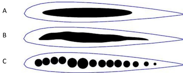
**Fig 8:** Various bladder configurations [G]
