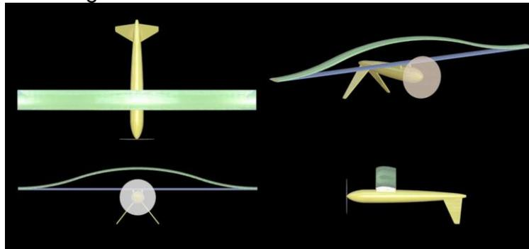
**Fig 6:** Different view of Buckled wing UAV [J]
