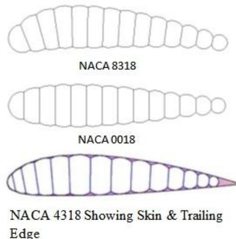
**Fig 9:** Inflatable wings [H]
