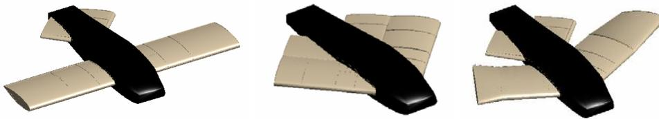
**Fig 1:** Wing morphing for loiter, dash and asymmetric maneuvering. [A]
