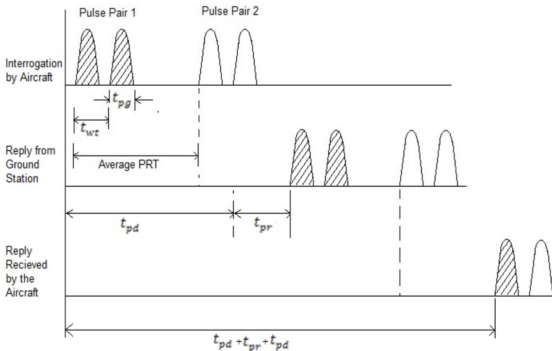
**Figure 1: DME Pulse waveform**
