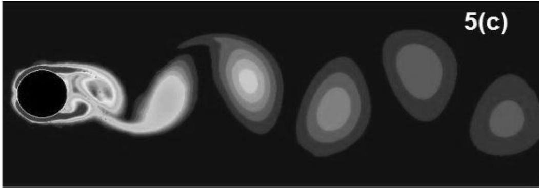
Fig 6: Vorticity distribution visible from the top view of the cylinder at (a) center plane, (b) 0.02 meter offset from center plane, (c) 0.04 meter offset from center plane.
