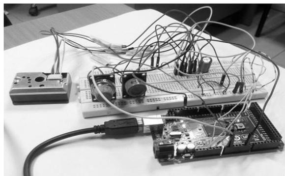
The MQ-9 gas sensor when subjected to the carbon monoxide produces output in the form of voltages that can be calibrated according to real world scenarios. It has a variable resistor on its body which can be used to calibrate the output voltage of the device. According to our scenario higher readings in the range (1-1000) tend to indicate higher levels of carbon monoxide.
