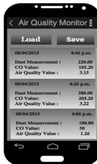
The device can be placed anywhere and data can be taken from anywhere within the Bluetooth's range. We opted to provide further convenience to the users of the device by developing the Android application which will receive the data from the device when connected. Figure 9 shows data being sent to the serial monitor of a computer having an Arduino development environment.
