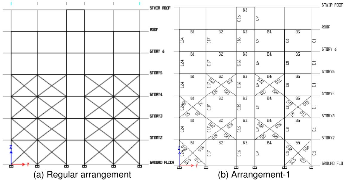
Figure 4: Elevation of building with X bracing type
