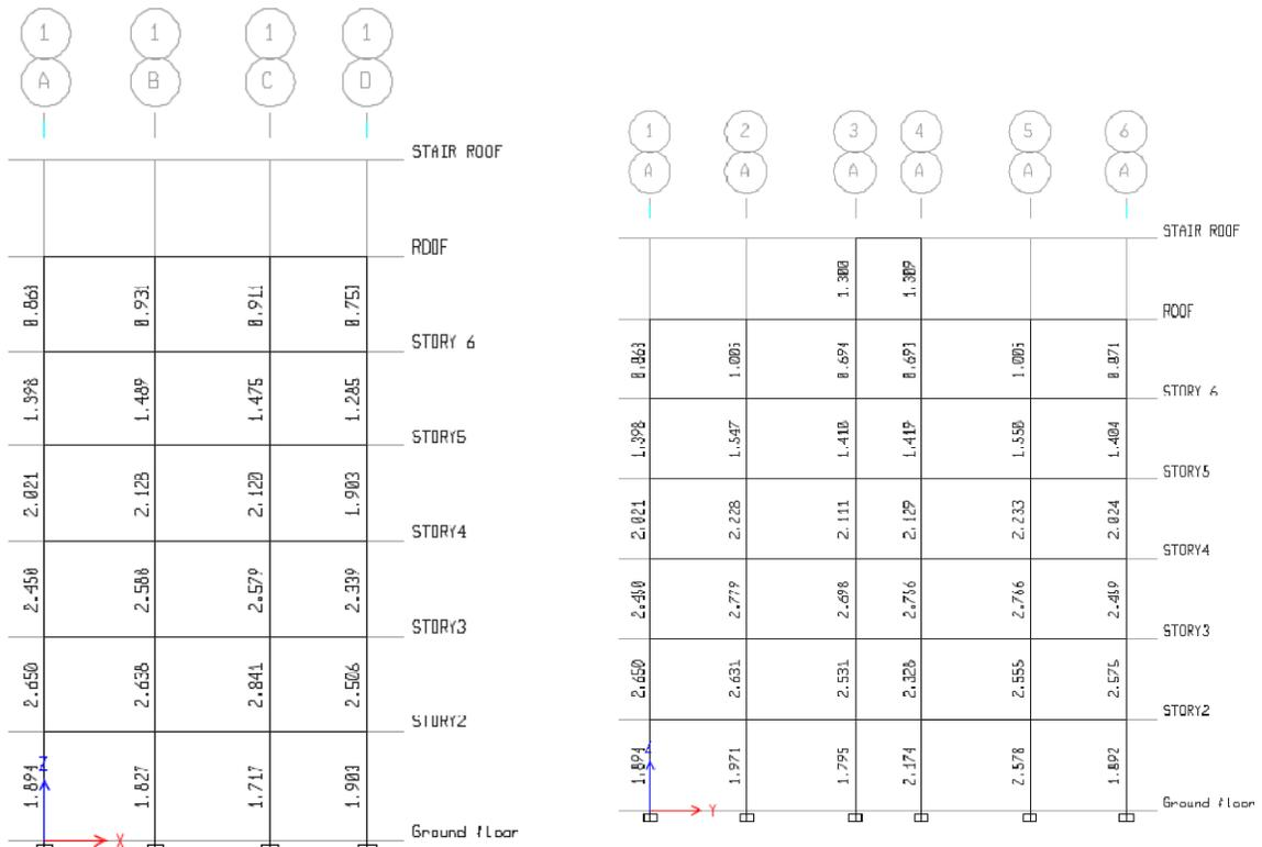
Figure 2: Column P-M-M ratio of frame 1-A-B-C-D and A-1-2-3-4-5-6
