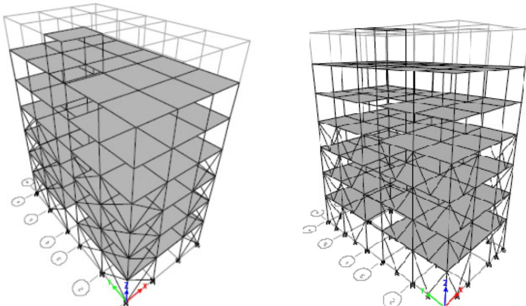
Figure 3: 3D modelling of the building with X type and V type bracing
