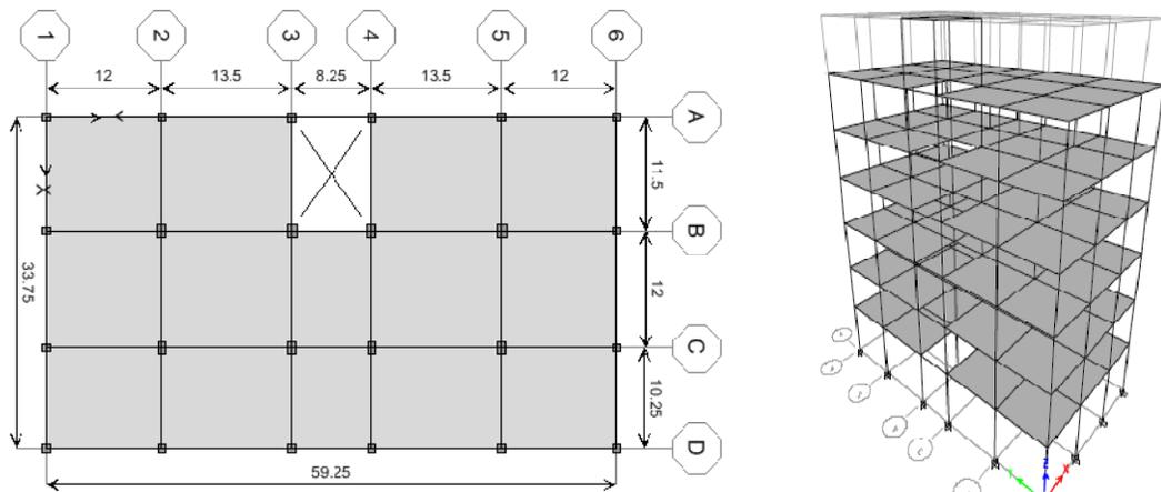
Figure 1: 3D finite element model of the building
