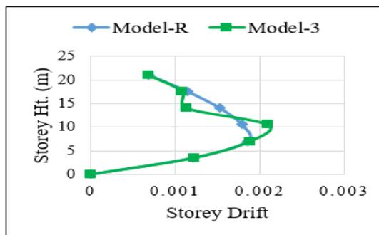
Figure 6. Storey drift of model-R and model-3
