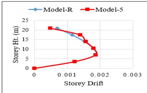
Figure 8. Storey drift of model-R and model-5
