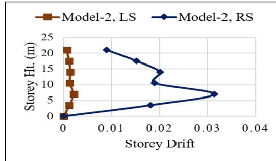
Figure 11. Model-2, Linear static (LS) vs. response spectrum (RS)
