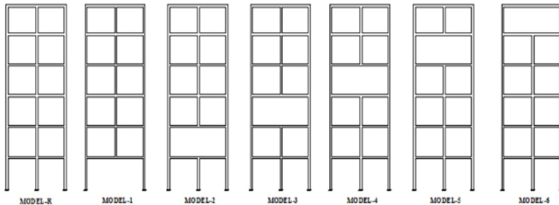
Figure 2: Base frame and different irregular models
