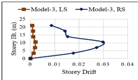
Figure 12. Model-3, Linear static (LS) vs. response spectrum (RS)
