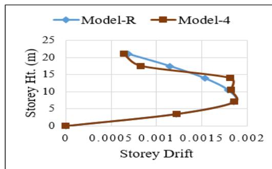
Figure 7. Storey drift of model-R and model-4
