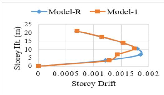
Figure 4. Storey drift of model-R and model-1
