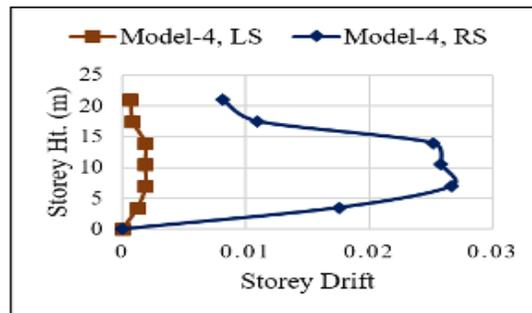
Figure 13. Model-4, Linear static (LS) vs. response spectrum (RS)
