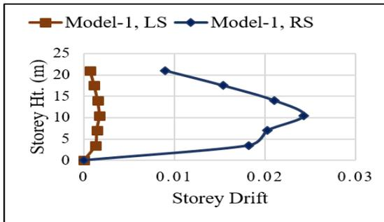
Figure 10. Model-1, Linear static (LS) vs. response spectrum (RS)
