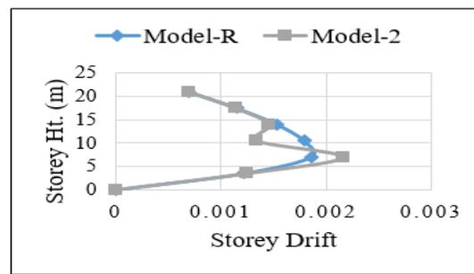
Figure 5. Storey drift of model-R and model-2
