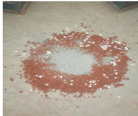
**Fig 2: Mixing of EPS beads with brick chips**
